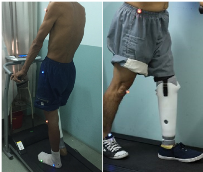
Figure 2. Gait Motion Analysis Sensor Placement. Left: Sagittal Left. Right: Sagittal Right.
